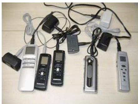
These devices were used to connect into the telephone exchange of a shopping mall to record all transmissions from the stores to the merchant's financial institution.
